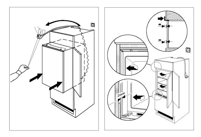
Fit appliance retaining screws
